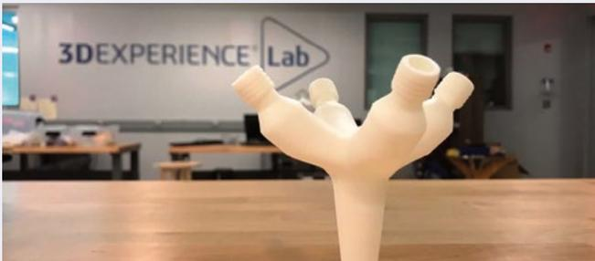
The **3DEXPERIENCE**® platform was used to optimize a flow splitter so that it could provide air to multiple patients at one time.
