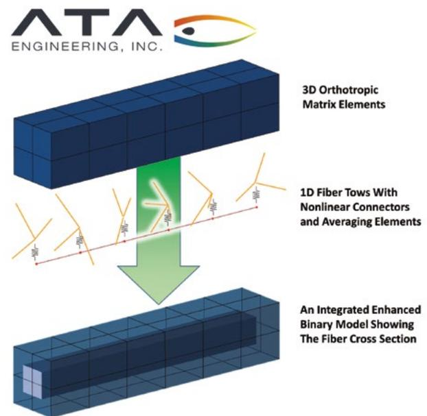
Figure 1. The EBM formulation for composite material architectures.
