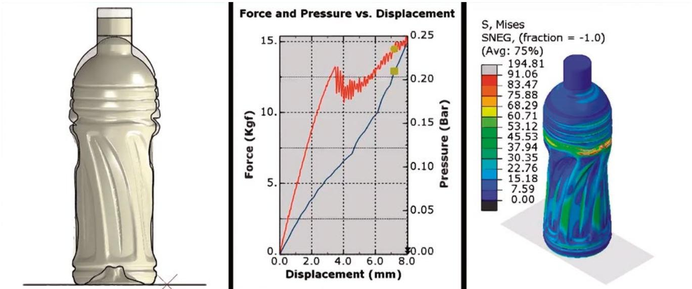
By leveraging a Virtual First Principal to test products virtually before performing any physical tests, PepsiCo ensures that new packaging will pass all requirements.
