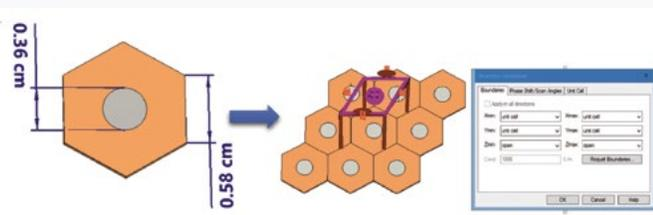
Figure 1. Unit cell structure; Floquet mode analysis of infinite array with the help of Unit Cell Boundary condition provided inside Frequency domain Solver.
