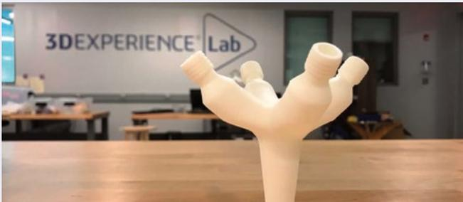
The **3DEXPERIENCE**® platform was used to optimize a flow splitter so that it could provide air to multiple patients at one time.
