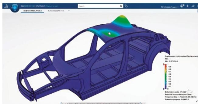
Figure 2: Initial roof design vibration mode shape
